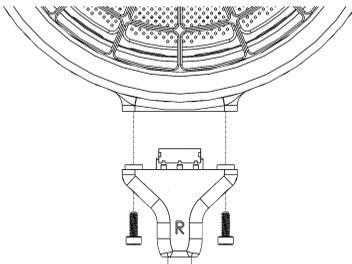
The headphone cable can be replaced by the owner. This connector is only meant to facilitate cable swapping and is not intended for daily cable changes.
