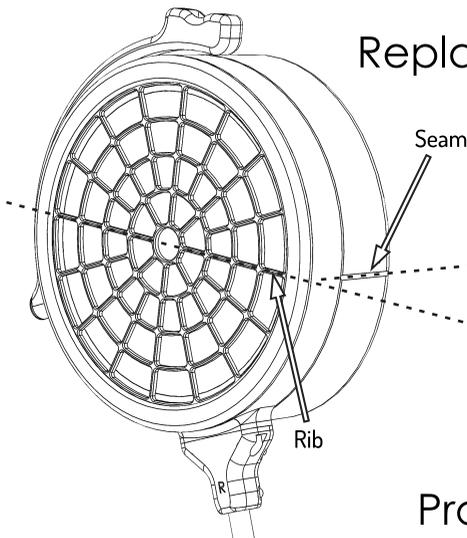
The ear pads are designed to be user replaceable. They pull off easily and have a notch in the plastic pad ring to assist installing a replacement pad. To put a new ear pad on slide the leather flange over the plastic ring completely.
