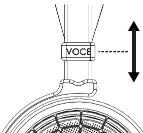
Adjust slider up or down on both left and right sides for proper fit.
