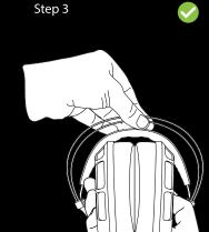
Push down on the headband wire while firmly holding both sides of the headphone with other hand. This will cause the headphone to fold in a controller manner.
